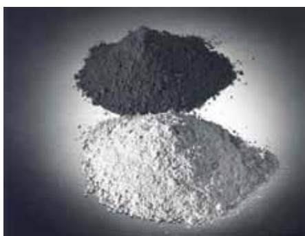
Figure 8c Silica fume, an industrial byproduct, is commonly used to replace cement in quantities from 5% to 7%.
