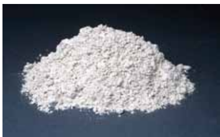
Figure 8b Slag cement is a cementitious material and a byproduct of the iron industry.
