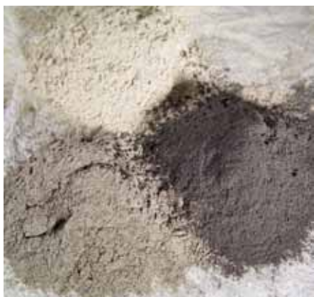
Figure 8a Fly ash, a byproduct of the electric industry, can be used as a partial replacement for portland cement.
